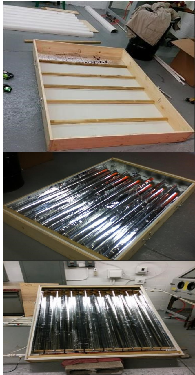
Figure 5. Steps used to fabricate the Solar Collector
